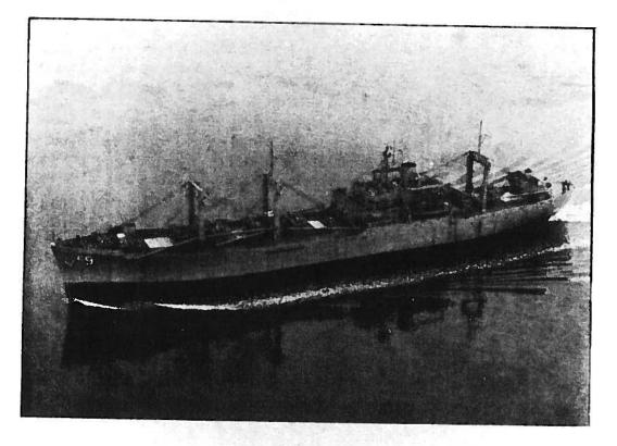
MAZAMA is a Lassen Class Ammunition Ship, built as an ammunition ship using C-2 hull plans. This vessel differs from earlier ships of her class in that these earlier ships (AE's 3,4,5 and 6) were first built as C-2 cargo vessels for the Maritime Commission and were later converted to ammunition ships.
